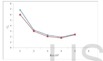
Fig 8. Comparison of Cd between with vortex and without vortex Generator
