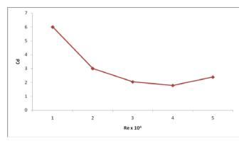
Fig 7. Reynolds number (Re) Vs Coefficient of drag (Cd) graph with vortex generator
