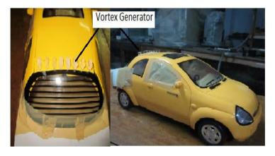
Fig 4. Experimental model of car with vortex generator
